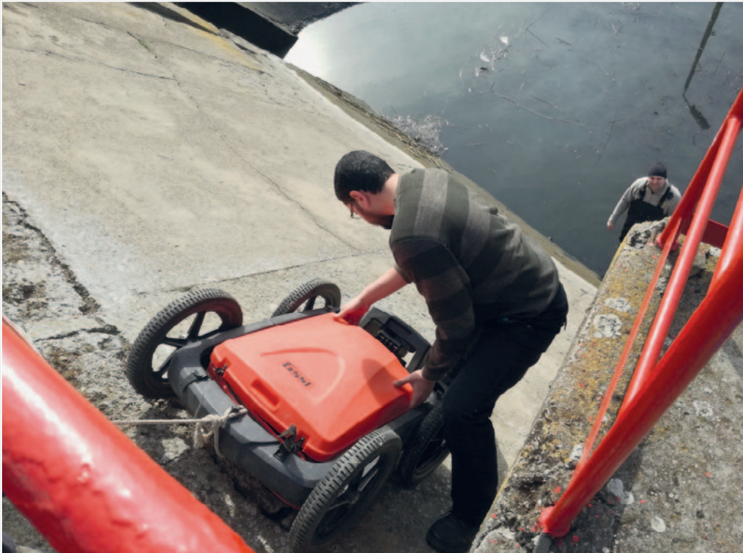
Performing a fracture assessment to detect leakage zones in the concrete.
