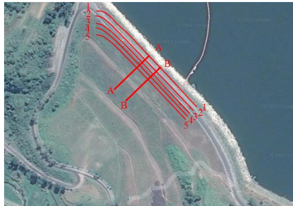
Fig. 2. ERT profile lines plotting on the body of the earth dam
