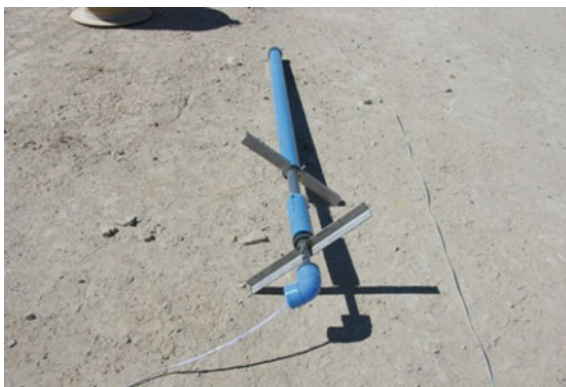
Fig. 31 Installation of long-gauge extensometers in the body of the tailing dam. Courtesy of Geomediciones
