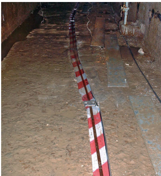
Fig. 22 Distributed strain sensing cable installed by clamping in the dam inspection gallery. The sensor runs along the length of the gallery and is therefore able to pick-up deformations generated by transverse cracks crossing its path. The blue temperature sensing cable installed along the strain cable is used for temperature compensation, but can also detect water ingress in the gallery by observing rapid temperature changes
