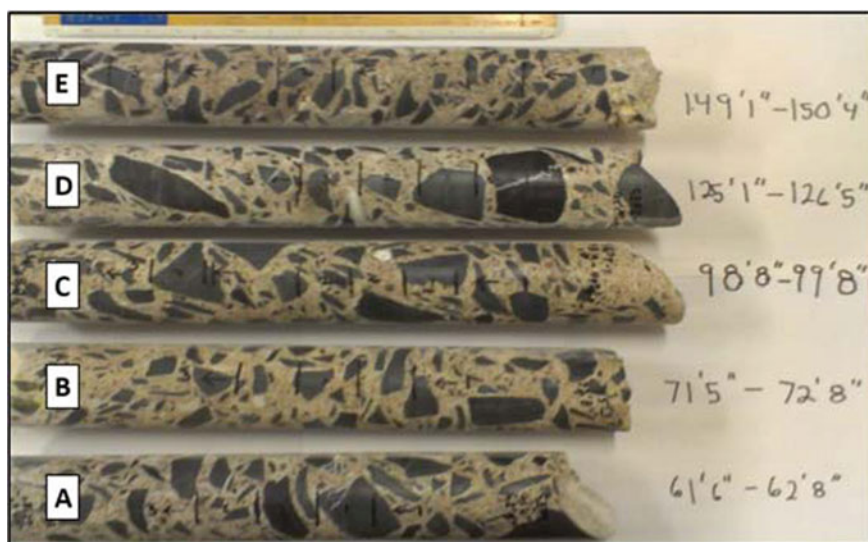
Fig. 6 Five concrete core samples (2.5" or 63.5 mm diameter) collected between depths of 20 and 45 m in borehole SEPI-1. Aggregate pieces are greywacke. Fractional porosities determined by hydrostatic weighing of three 30 mm thick disks from each sample varied from 0.11 to 0.16 ( \pm 0.02 )
