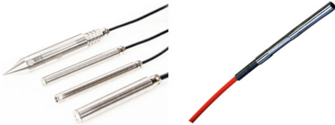
Fig. 4 Fabry-Perot piezometer with conventional (left) and miniature (right) packaging
