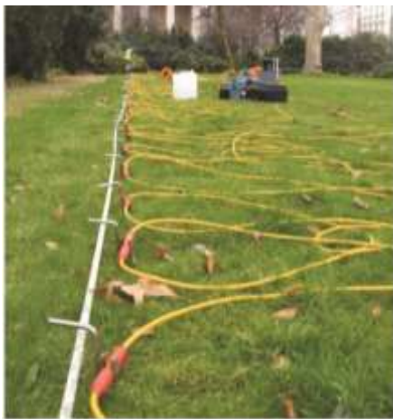
Figure 6- ERT electrode setup (RSK Geophysics, 2016)
