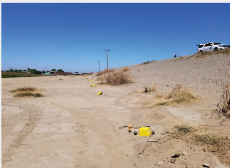
Image showing data collection during a passive seismic survey in the Sacramento Delta.
