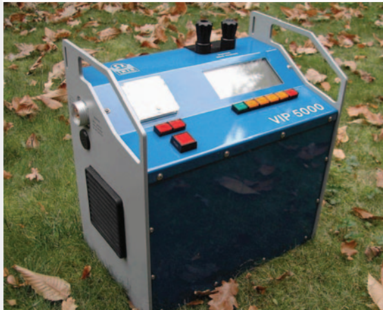
High power VIP 5 kW transmitter.
