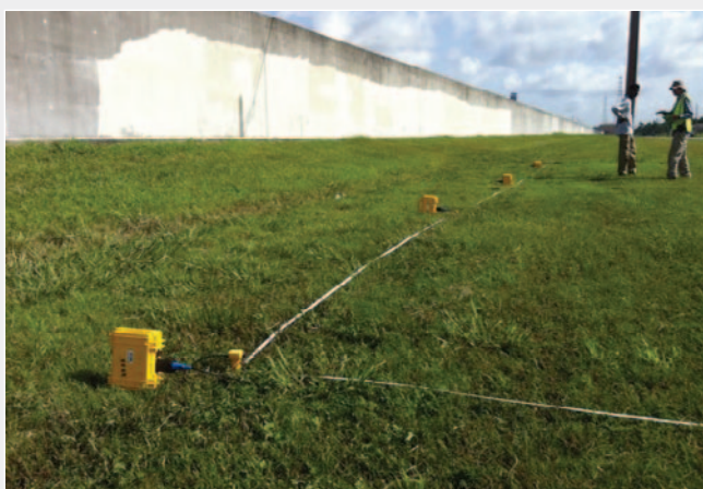
Image shows a line of Atom Wireless Seismographs at the location of the levee rupture and the new levee (concrete wall).
