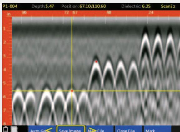
*This data image example is from a 2.7 GHz frequency antenna showing a series of hyperbola. These hyperbolas correspond to pieces of rebar located at different depths ranging from 1 – 5’.*
