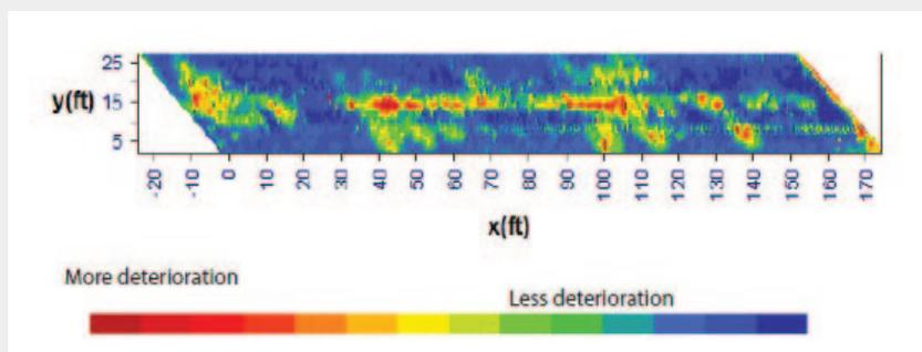
*GPR software denoting areas of concrete deterioration.*
