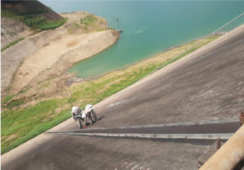
*Using the GSSI StructureScan Mini XT GPR system for a concrete dam condition assessment.*
